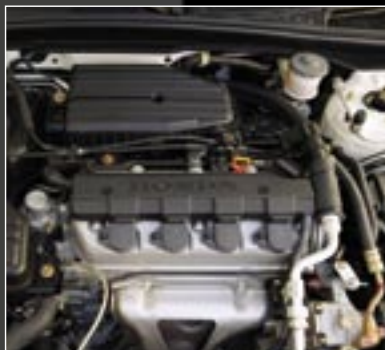
The GX uses a 1.7-liter natural gas engine.
