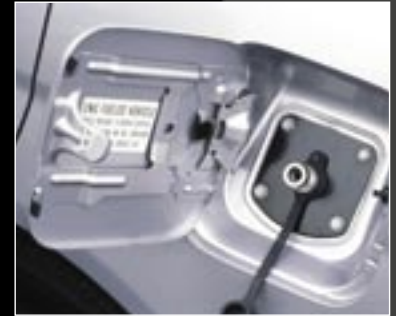
Gaseous fueling is at the standard location.
